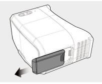
2. Slide the Wi-Fi DVR Module on to the ARX-500 FPV Goggles.
