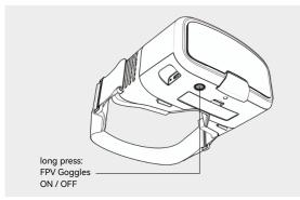
Once the ARX-500 FPV Goggles is switched on, Wi-Fi DVR will emit a long "beep" sound 20 seconds later, indicating the boot sequence is complete and it's ready for recording.
